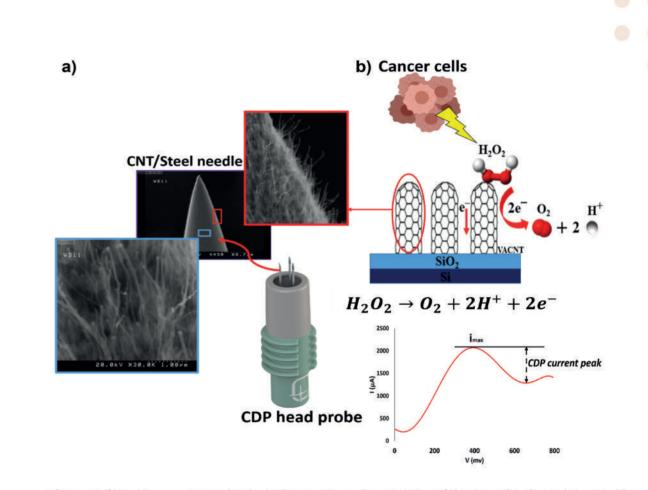
a) Image of the CDP Margin HeadProbe in the margin mode, consisting of three needle electrodes coated by multi-wall carbon nanotubes (MWCNTs).
